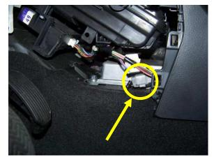
If water is found, diagnose the origin of the water and repair as necessary.
