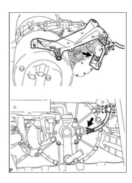
(b) Disconnect the shift control actuator connector and speed sensor connector.
