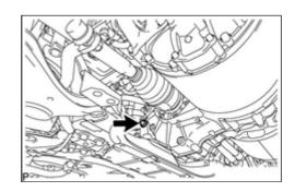
(b) Operate the powertrain lift table or equivalent and slowly remove the electric vehicle traction motor assembly from the vehicle.
