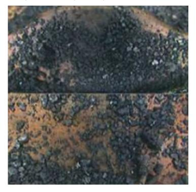
Carbon deposits are not abnormal inside combustion chamber, but some of the existing fuel additives in the market can affect deposits concentration in terms of amount and size. Once those deposits flow through the exhaust valves, the biggest ones could remain between the valve and the valve seat creating a gap. This gap causes lack of compression and consequently, difficulties to start the engine.
