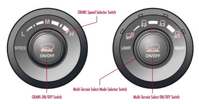
Another system new to 4Runner but similar to Land Cruiser is CRAWL Control. This system automatically controls engine output and braking force to maintain a manually-selected speed between 1 and 3 miles per hour. This allows the driver to focus on steering when driving in difficult terrain. The system is turned ON/OFF and one of five set speeds is selected using controls located in the overhead console.
