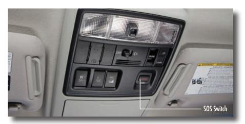
The 2010 4Runner adds even more peace of mind with an optional Safety Connect system. As on other Toyota models, this system provides emergency call services through a cellular network. The system includes an SOS Switch in the map light assembly and a Back-up Battery located behind and to the left of the glovebox. Always refer to the Repair Manual for diagnosis and repair of the Safety Connect system.
