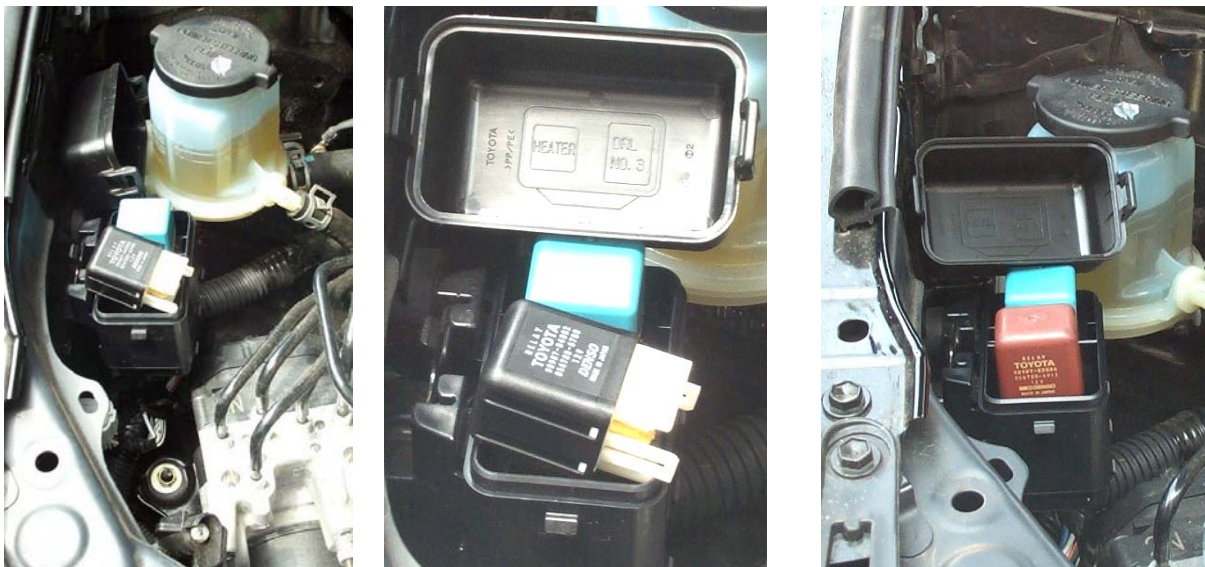
Location DRL No.3 on RX330 "Native" (OEM) Relay DRL No.3. "New" Relay No.3 (DRL is disable)
