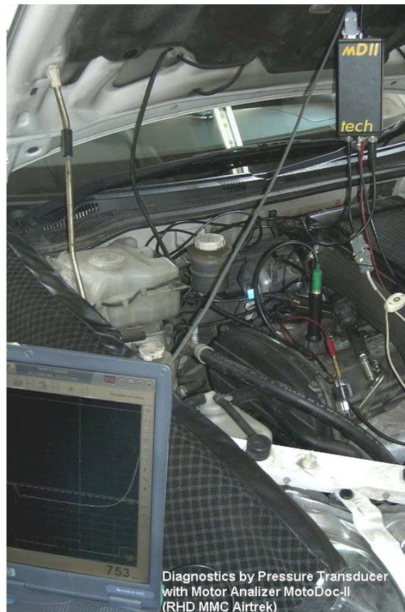
Diagnostics by Pressure Transducer with Motor Analyzer MotoDoc-II (RHD MMC Airtrek)
