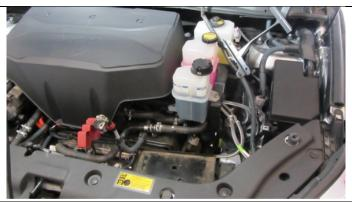
2012-2014 Toyota RAV4 EV – **12 volt battery removal supplement** - Drill a 5/8" or 3/4" (14-18mm) diameter hole using "Forstner" or other drill bit into the plastic panel shown to expose the M6 bolt (10mm hex head bolt) underneath. The recommended drilling location is cetered directly below the word "VENTILATEURS", on the upper portion of the Japanese character aligned below the letter "R"
