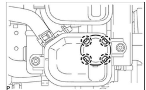
(c) Remove the battery reservoir tank cap.
