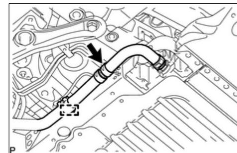
(e) Disconnect both the No. 7 and No. 8 EV battery hoses, and drain the coolant.
